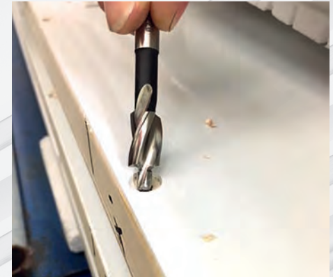
Original pilot counterbore for countersinking fiberglass roofs made of HSS.
