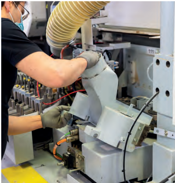
To adjust the tool, the machine operator simply opens the hood. The tool does not have to be removed for adjustment.
