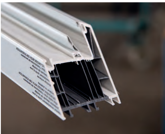
Schock Fensterwerk requires clean and burr-free chop cuts, even when the seals are already installed. Schock Fensterwerk requires clean and burr-free chop cuts, even when the seals are already installed.
