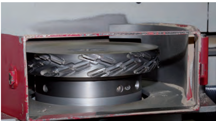
The diamond-tipped cutting edges with 70° shear angle on the p-System tool can be seen clearly.
