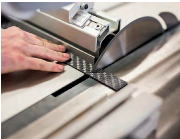
Cutting CFRP with the diamond-tipped LEUCO nn-System DP Flex saw blade
