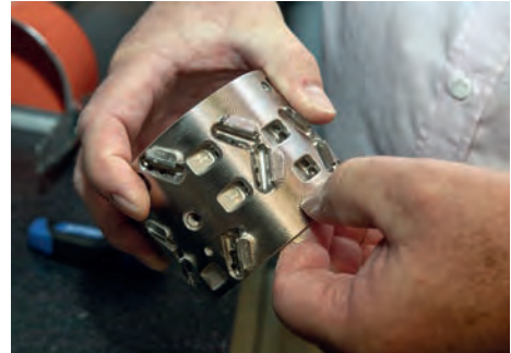
The pair of holes in front of the cutting edges is an Airstream feature. The holes guide the air flow with the chips directly into the dust extraction. In addition, they reduce air turbulence; the machine is noticeably quieter.
