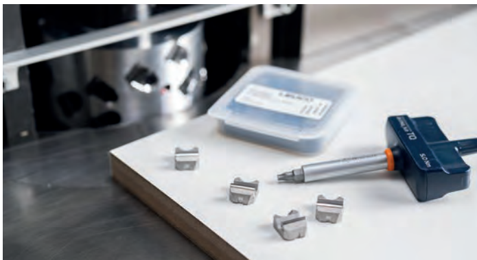
The jointing cutter for MAN feed is available with a 125 mm diameter, a cutting width of 43 mm, and 12 segments or, in an alternative model, with 64 mm and 18 segments. What makes the SmartJointer stand out is the fact that the diameter remains consistent even after replacing the cutting edges so that the machine does not have to be recalibrated or adjusted. Also, potentially damaged or heavily worn cutting edges can be replaced individually in place, thus extending the service life.
