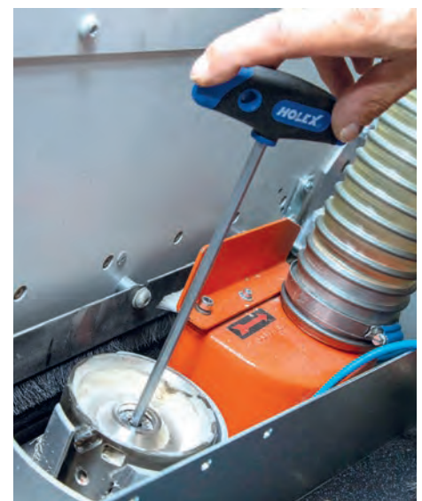
High precision despite simple handling: The DIAMAX AirStream HSK 32 F jointing cutter from LEUCO can be clamped in the machine quickly with an Allen key.
