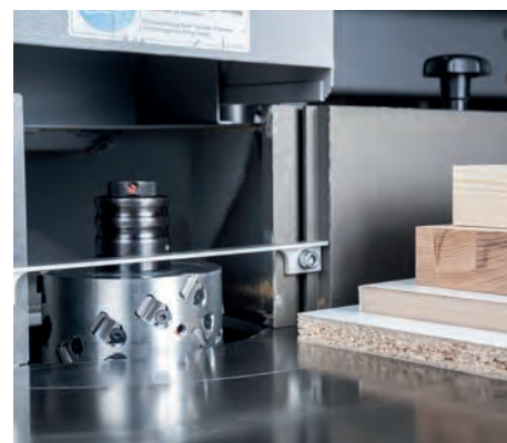
The 35° axis angle enables the diamond-tipped SmartJointer to joint solid wood and woodbased materials without chipping. The diamond tips also mean longer edge lives.
