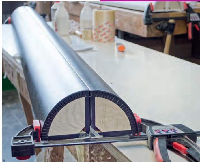
Two curved quarter-segment columns with a particularly uniformly curved surface
