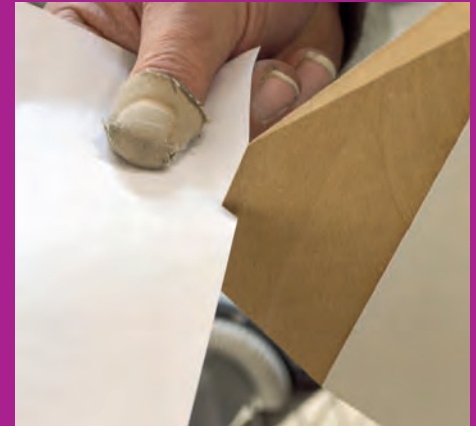
The miter just cut effortlessly slices a sheet of paper
