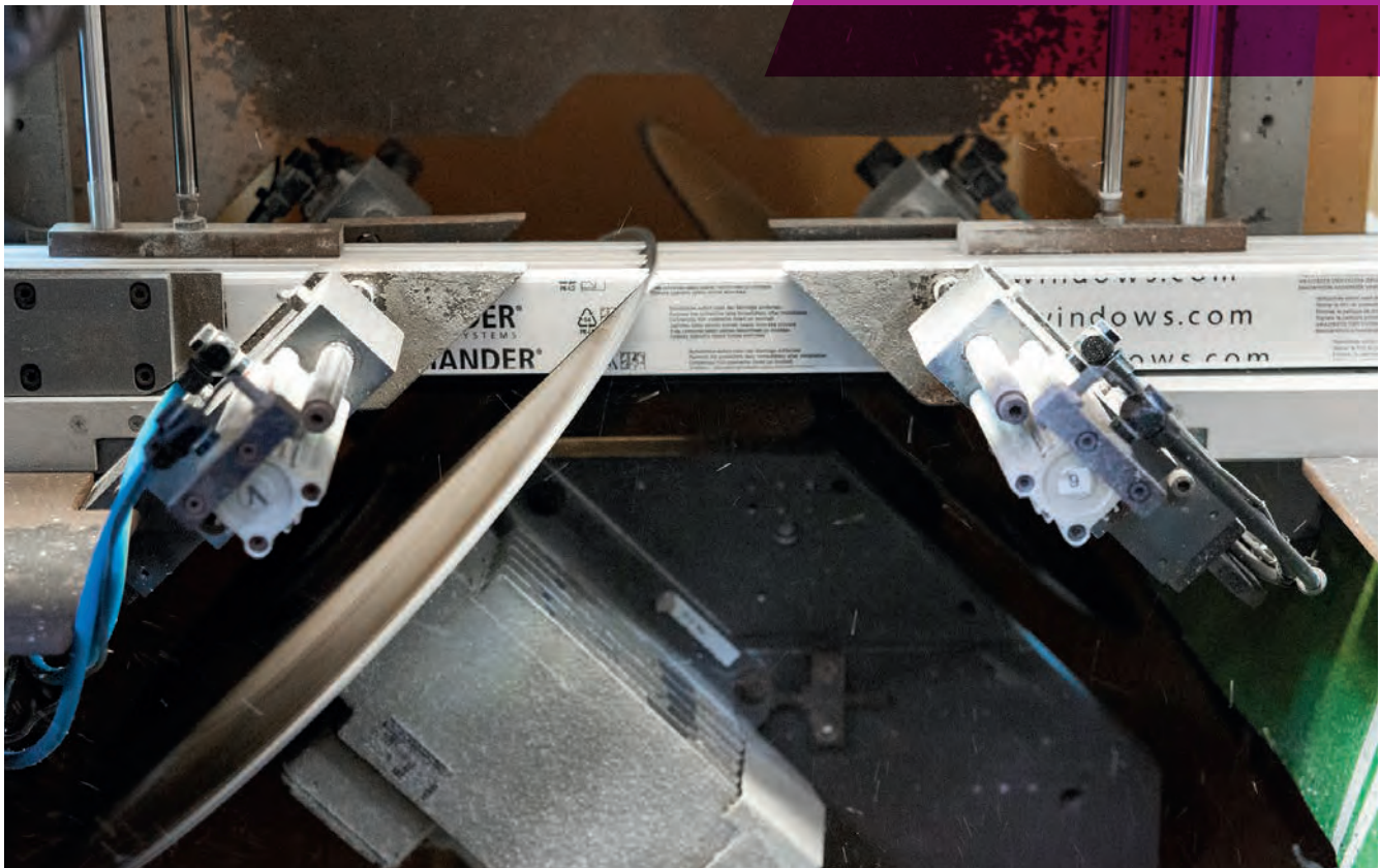
Schock Fensterwerk cuts window profiles using standard and modified LEUCO saw blades with long service lives.
