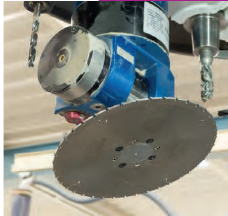
... and hangs it in the tool magazine of the 4-axis CNC
