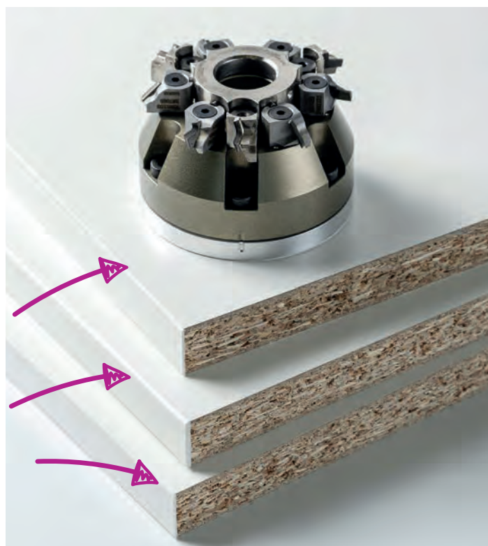
Three profiles can be changed in a matter of seconds with the new multi-profile shape cutter for edge banding machines from OTT.
