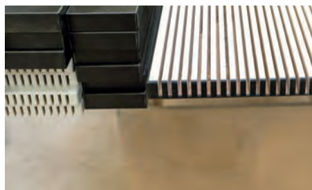
The joinery also uses the nn-System DP flex on the panel saw for grooving bending panels
