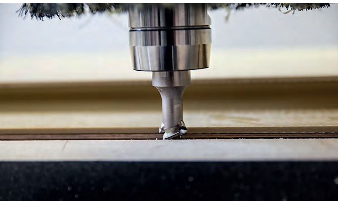
Cut aramid (e.g. Kevlar®) cleanly with LEUCO p-System tools
